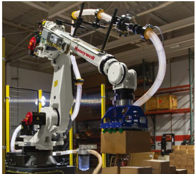
AI software and related vision and perception capabilities provide this depalletizer with its intelligence and ability to handle variation.
